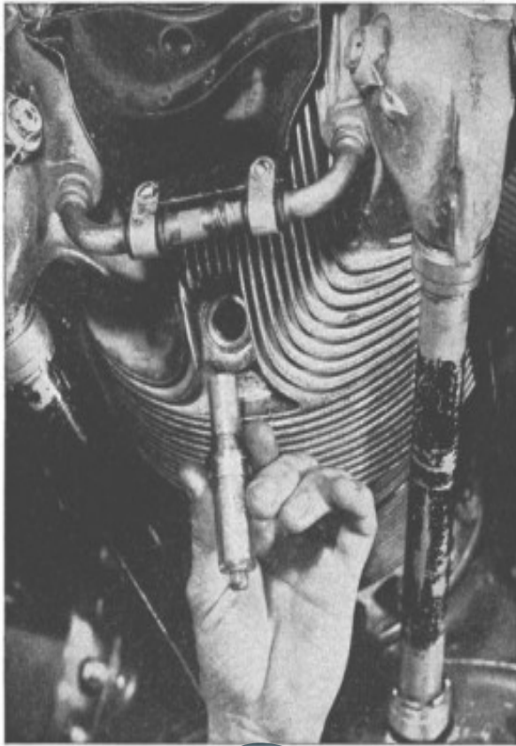
Figure 85. Installing dehydrating plug in the engine cylinder.
