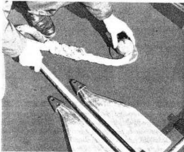
Figure 4—Cap in Place on Deck Pipe
