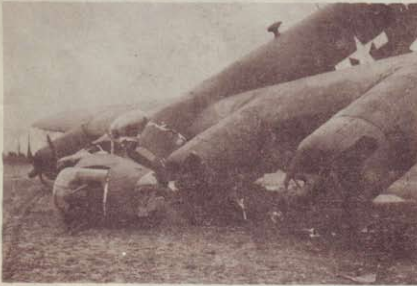
THE PILOT OF THIS AIRCRAFT MIGHT HAVE BEEN A GOOD PILOT, BUT THIS IS WHAT HAPPENED WHEN PILOT ATTEMPTED TO " LAND DOWN-WIND "
