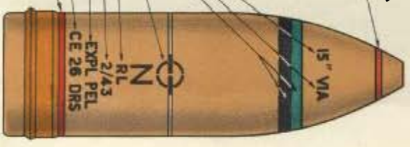
TYPICAL NOSE FUZED SHELL HE FILLED TNT
