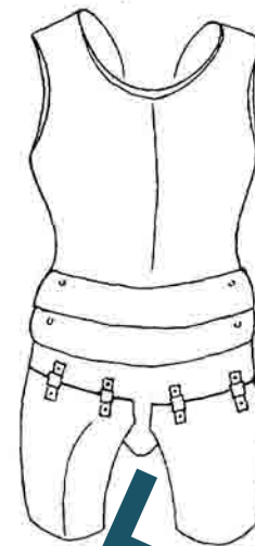
Figure 191.—A body armor for sentinels, designed to protect the wearer from chin to knees, with breastplate proof to a service rifle bullet at 40 yards, 2,750 foot-seconds. The weight of this armor, without thigh guards, is 24\frac{1}{2} pounds, but this is evenly distributed.
